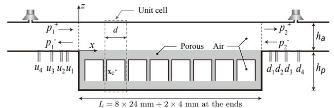
FIG. 2. A 2D schematic view of the experimental setup. The measured sample, of length  $L = 200$  mm, contains 8 unit cells.  $\mathbf{x}_c$  is the center of the rigid inclusion.
