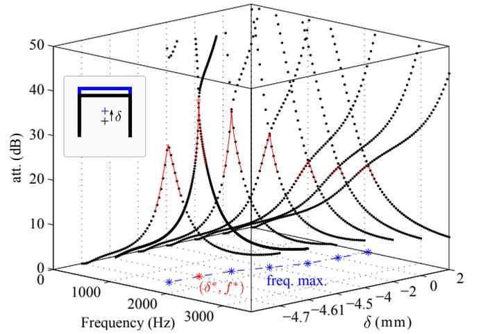
FIG. 6. Mode attenuations for the lower two Bloch modes as a function of frequency at different inclusion positions  $\delta$ .  $\delta$  is positive when the cylinder centre  $\mathbf{x}_c$  is moved above the center of the cell, and negative when  $\mathbf{x}_c$  is moved below the center of the cell.
