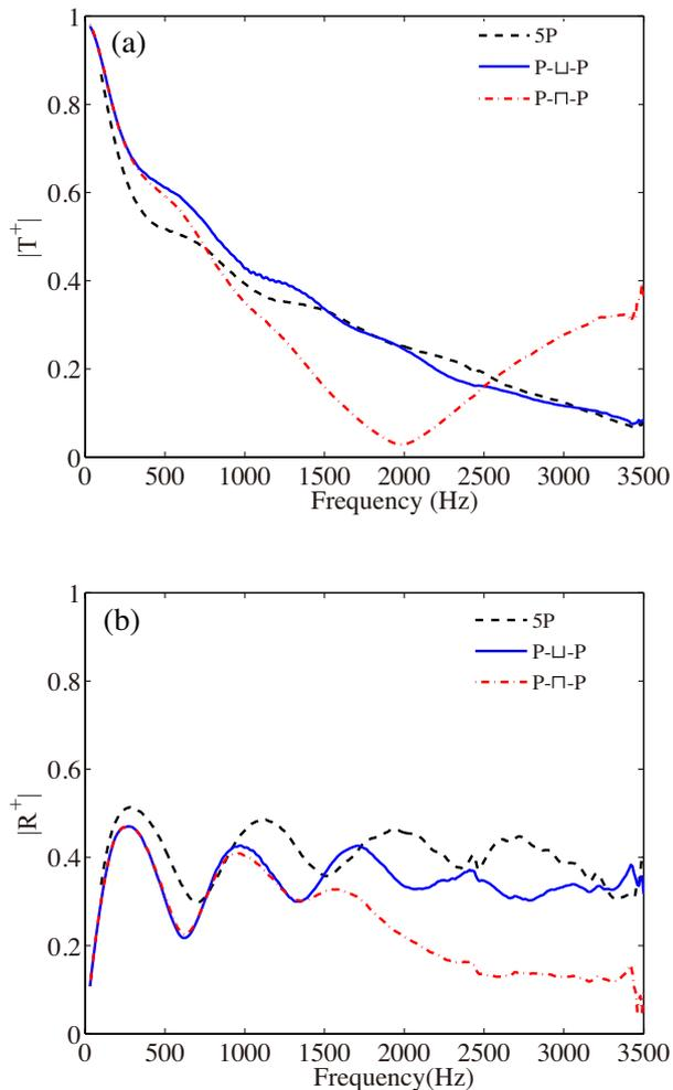
FIG. 4. Measured scattering matrix coefficients for the three configurations: 5P (---), P-⊥-P (—), and P-⊓-P (---). (a) Absolute value of transmission coefficient  $T^+$  and (b) absolute value of reflexion coefficient  $R^+$ .
