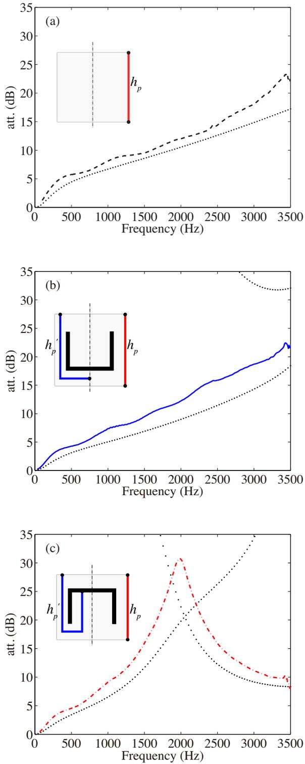
FIG. 5. Comparisons between the Bloch mode attenuation computed using Eq. (9) ( $\cdots$ ) and the measured transmission loss ( $- -$ ,  $-$ ,  $- -$ , respectively) with 8 unit cells for the configurations: (a) 5P, (b) P-L-P, and (c) P- $\Pi$ -P. The inserted schemes in (b) and (c) show the *effective* heights  $h'_p$  of the latter two configurations.
