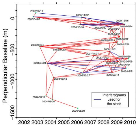
**Figure S-2:** Dates of image acquisitions as a function of perpendicular baseline. Red segments show the interferograms that have been calculated, among which blue segments show the interferograms used for the stack.
