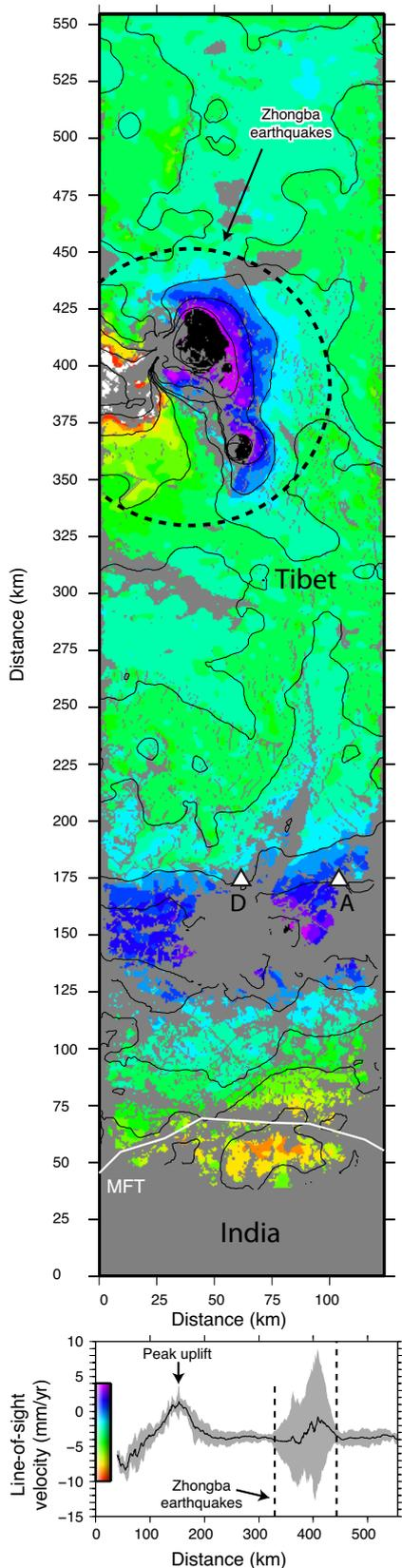
**Figure S-7:** Stack obtained by summation of unwrapped interferograms of Figures S-5 and S-6. Note that the average velocity has been calculated from pixels that have been correctly unwrapped for all 14 interferograms. Bottom panel shows a cross-section for a profile crossing the image along the satellite heading direction (azimuth direction), with the black curve corresponding to average line-of-sight velocity on each line, and the grey envelope showing  $1\sigma$  standard deviation.
