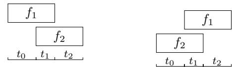
(a) A possible trace of execution for f_1 and f_2 (b) Another trace of execution
