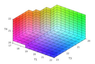
Fig. 2. Visualization of the domain  $dom(C_{\sigma}^2)$  of the safety controller for subsystem  $\sigma = 4$  of  $S_c^2$ . Each axis is associated with one component of the RGB color model to facilitate the visualization of depth.
