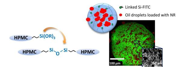
Scheme 1: This scheme represents the protocol of preparation of FMGs and BPMGs based on the solgel reaction and a templating emulsification process. The pH and the temperature are the main parameters that control the chemical cross-linking reaction, leading to formation of Si-O-Si bonds. The Si-HPMC network could be functionalized with a model molecule, such as Si-FITC in FMGs. Oil compartments for lipophilic molecules encapsulation, were trapped in the BPMGs.
