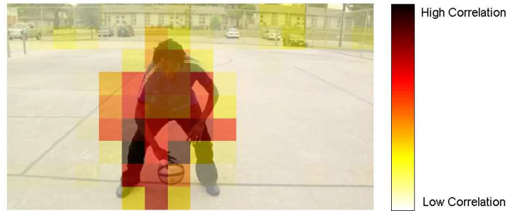
Fig. 2: CCA Illustration: Heat map showing correlation between video image regions and audio. Black squares indicate highest correlation.
