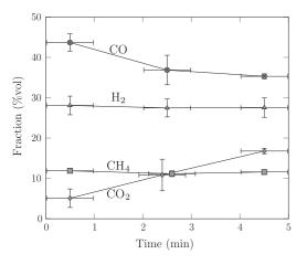
**Fig. 7.** Gas composition downstream the tar condensing device for the reference case (9 %wb, end grain). Triangle: H<sub>2</sub>, circle: CO, diamond: CO<sub>2</sub>, square: CH<sub>4</sub>.
