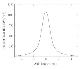
Fig. 2. Incident heat flux on the sample surface.
