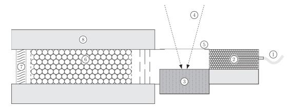
**Fig. 1.** Schematic of the reaction chamber. (1) Nitrogen inlet, (2) porous medium, (3) sample, (4) incident heat flux, (5) quartz window, (6) tar condensing device, (7) cotton trap, and (8) insulating material. Radiometer: not shown.
