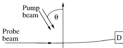
FIG. 7. Principle of the measurement of the directional absorptivity. The detector  $D$  measures the angular deviation of the probe beam (HeNe laser). The pump beam is a  $\text{CO}_2$  laser ( $\lambda = 10.6 \mu\text{m}$ ).
