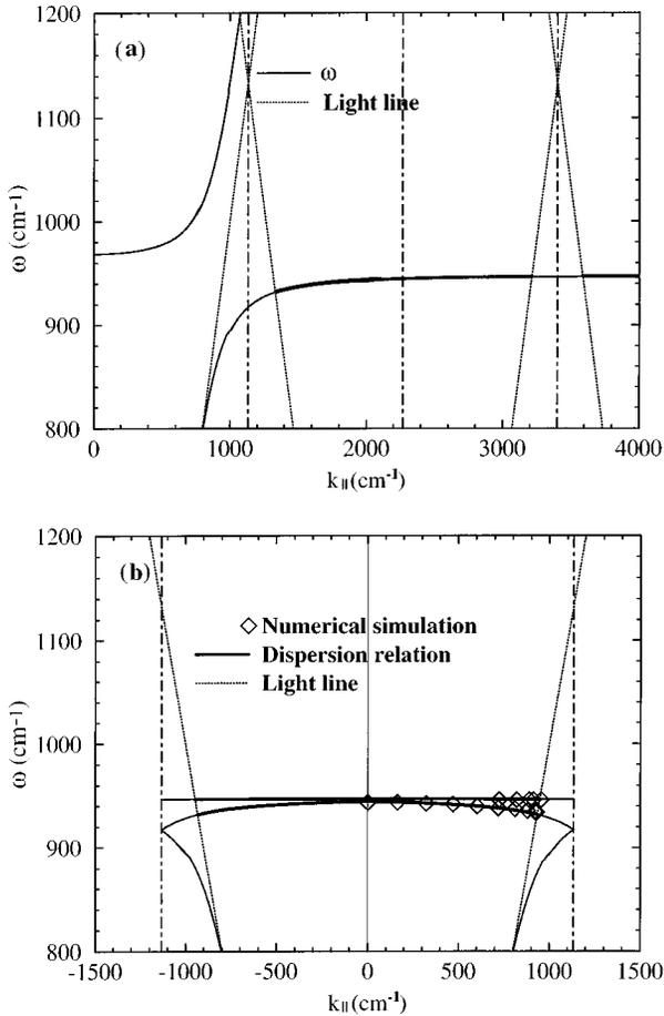
FIG. 2. Dispersion relation of a surface-phonon polariton on a smooth grating. (a) Extended zone scheme. (b) Reduced zone scheme.
