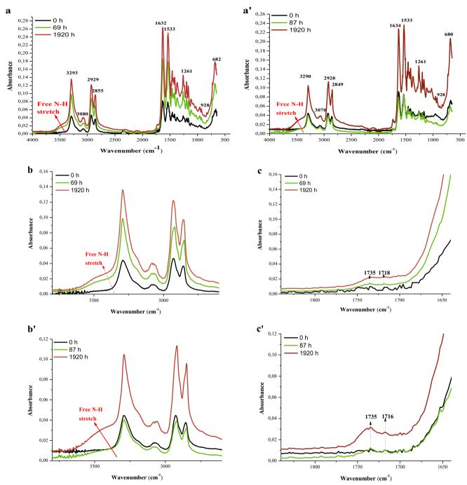
Fig. 8 Infrared spectra (a) of PA6 and PA6GF30 (a') submerged in distilled water for different conditioning times, (b,b') from 2600 to 3800 cm<sup>-1</sup> and (c,c') in the carbonyl area
