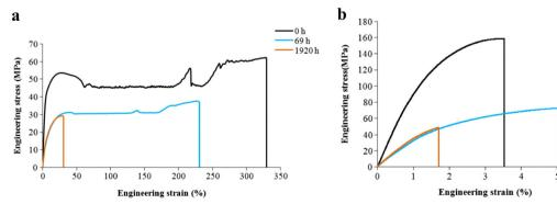
Fig. 9 Engineering stress-strain curves of (a) PA6 and (b) PA6GF30 at different conditioning times in distilled water at 90 °C
