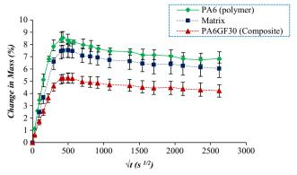
Fig. 1 Water absorption in PA6 and PA6GF30 fully immersed in distilled water at 90  $^{\circ}$ C for 80 days
