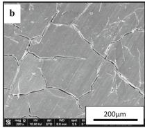
Fig. 4 Yellowing and surface observations of PA6 (a) and PA6GF30 (b) after thermal ageing for 80 days at 90 °C
