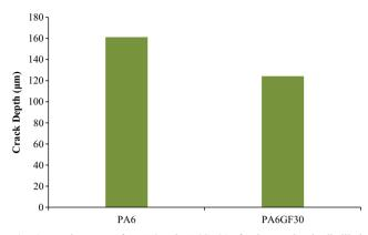
Fig. 6 Depth average for PA6 and PA6GF30 after immersion in distilled water a 90  $^{\circ}\text{C}$  for 80 days
