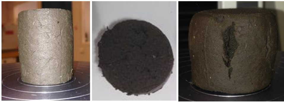
Figure 6: (a) Non-fractured sludge sample after compression test; (b) tested sludge sample cut into slice for internal crack detection: no internal fracture observed; (c) fractured sludge sample after compression test
