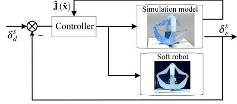
Fig. 1. The implementation of the open-loop controller. At each sampling time,  $\hat{\mathbf{J}}(\hat{\mathbf{x}})$  is computed from the simulation model and is used for the computation of control input for both the simulation model and soft robot.
