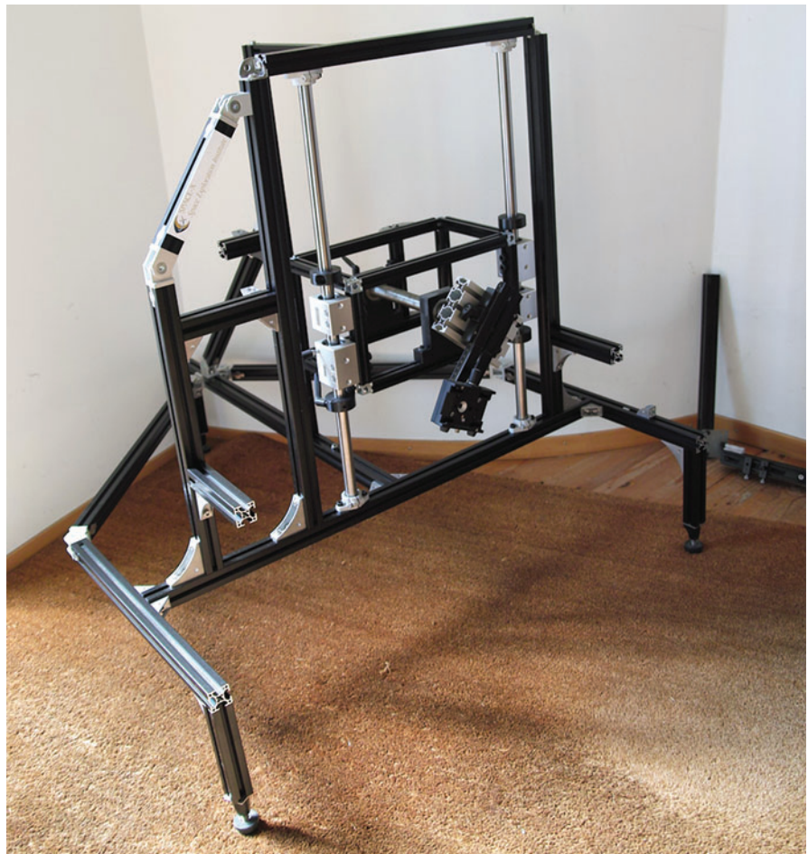
FIG. 17. Geometric drill simulator corresponding to the ExoMars 2020 Rover mission (scale 1:1) built at the Space Exploration Institute premises.
