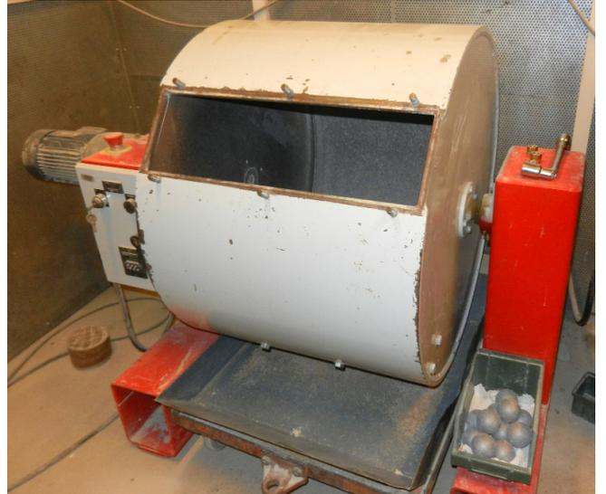
**Fig. 2** Picture of the Los Angeles testing machine used in this work.
