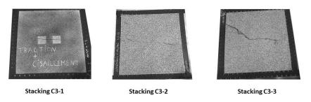
Fig. 17. Final failure pattern for combined tension and shear loading.
