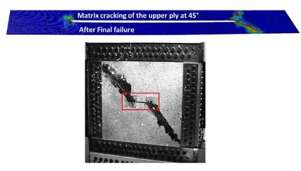
Fig. 29. Final failure for shear test, double thickness, comparison between experimental and numerical result.
