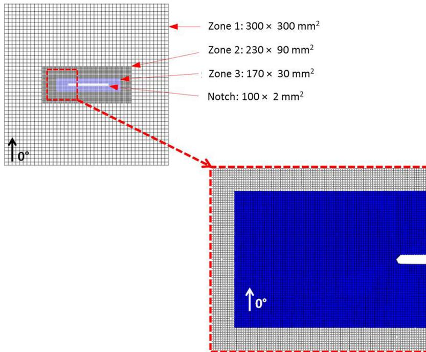
Fig. 21. Abaqus Mesh for analysis of VERTEX tests.
