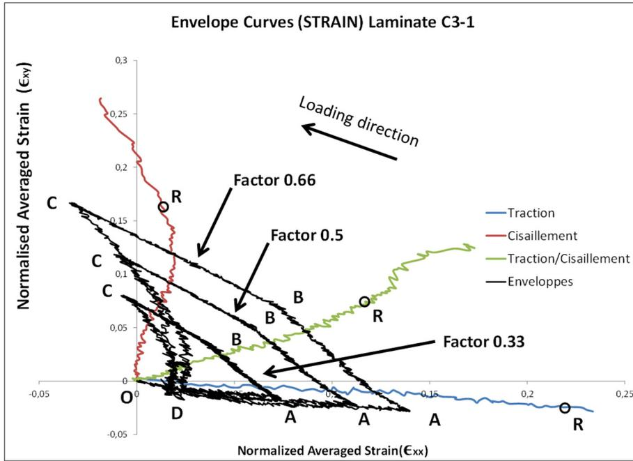
Fig. 32. Envelope tests in the strain space.
