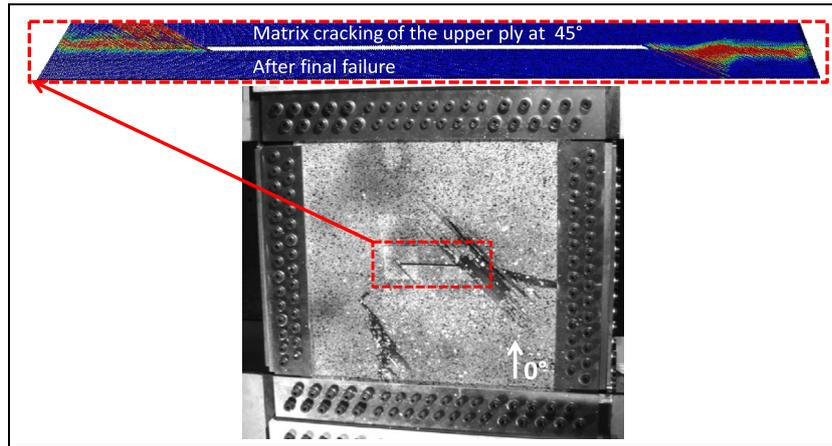
Fig. 25. Failure pattern: numerical vs experiment.
