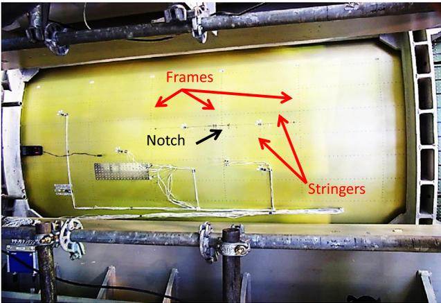
Fig. 1. Typical "Two-bay crack" test (Courtesy of Airbus).
