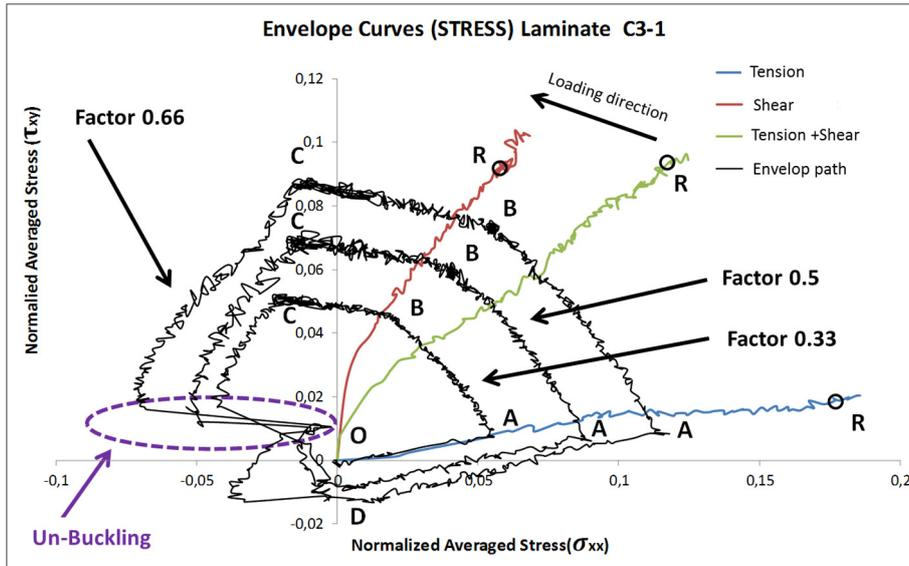
Fig. 33. Envelope tests in the stress space.
