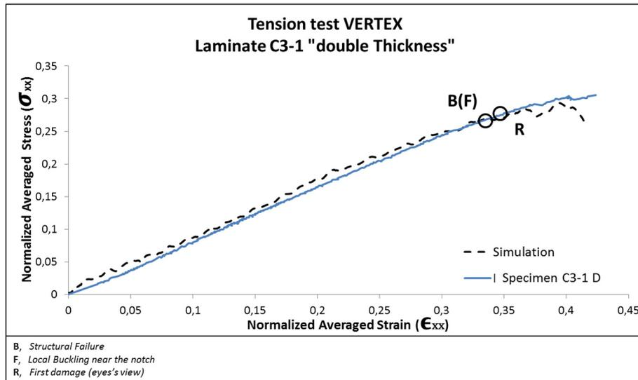
Fig. 22. Experimental/numerical comparison for VERTEX tension test.
