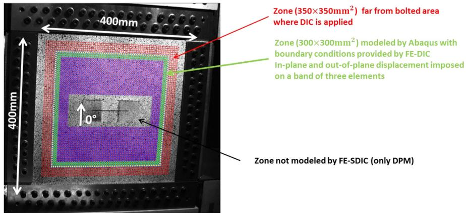
Fig. 20. Method of exchange of boundary conditions between FE-SDIC and numerical model.
