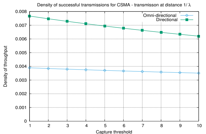
Fig. IV.7. Density of successful transmissions when the carrier sense detection threshold is optimized versus T . ( \lambda = 0.1 , r = 10 , T = 10 and \beta = 2 ).
