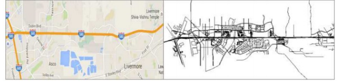
Figure 6. San Jose (California) urban area (left) exported to a VANET network topology by using MOVE/SUMO (right).
