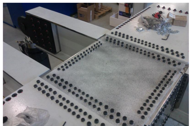
Fig. 15. (a) View of the hidden side of the aluminum test piece with three strain gauges oriented at 0^\circ , 45^\circ and 90^\circ . (b) View of the specimen bolted on the VERTEX device.
