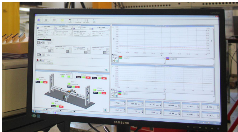
Fig. 8. Monitoring screen for actuators.
