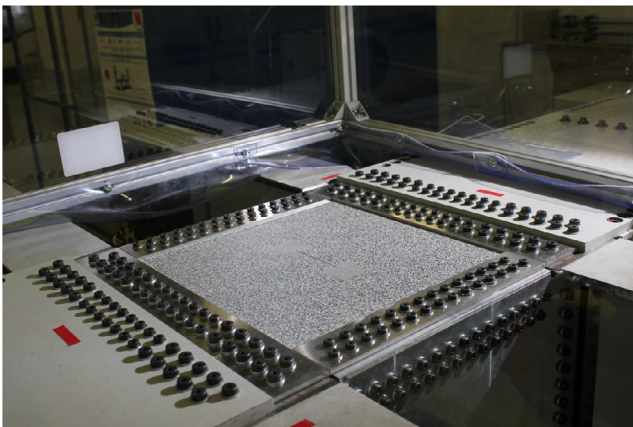
Fig. 10. Detail of a specimen bolted onto the upper part of the central box of the VERTEX test rig.
