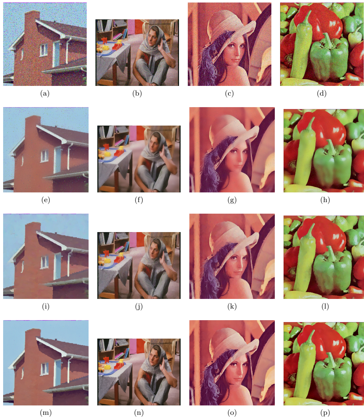
Figure 10. Visual illustration of edge-preserving filters on images contaminated with salt and pepper noise. BF erases some object boundaries while TF and order-based approximation yield similar results. (a), (b), (c), (d) Salt and pepper noisy images (e), (f), (g), (h) Bilateral Filter ( \sigma_{color} = 100 , \sigma_{space} = 10 ) (i), (j), (k), (l) Tree Filter ( \sigma = 10 ) (m), (n), (o), (p) Order-based multi-tree truncation ( \sigma = 10 , N = 100 )
