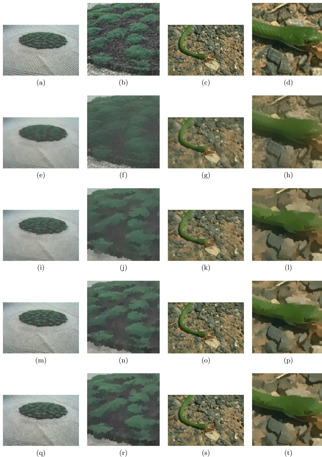
Figure 9. Subtle differences of the performance of TF vs our multi-tree approximations of UMSTF on BSDS500 [3] images are illustrated. (a), (b), (c), (d) original images (e), (f), (g), (h) Bilateral Filter ( \sigma color = 100, \sigma space = 10) (i), (j), (k), (l) Tree Filter ( \sigma = 10 ) (m), (n), (o), (p) Depth-based multi-tree truncation ( \sigma = 10 , depth = 15) (q), (r), (s), (t) Order-based multi-tree truncation ( \sigma = 10 , N = 100 ). In the second and fourth columns, observe the green patches and the snake's eye respectively. The leaks are more prominent in TF when compared to our approximations.
