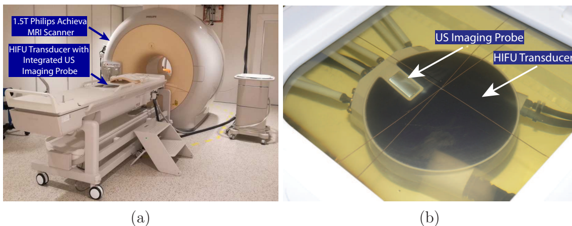
Figure 1: The custom-built HIFU system developed at our institute, which can provide MR and/or B-mode US guidance. (a): Overall setup. (b): The HIFU transducer together with the integrated US imaging probe.
