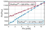
Fig.3. Bidirectional Pin/Pout vs Pin for the Si<sub>0.1</sub>Ge<sub>0.9</sub> waveguide.
