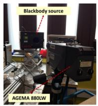
Figure 5: Test set-up for calibration of IR camera with the optical filter at 7.6 µm
