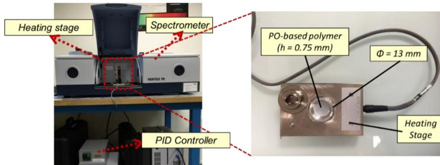
Figure 3: The test set-up for temperature-dependent bi-directional transmittance measurements
