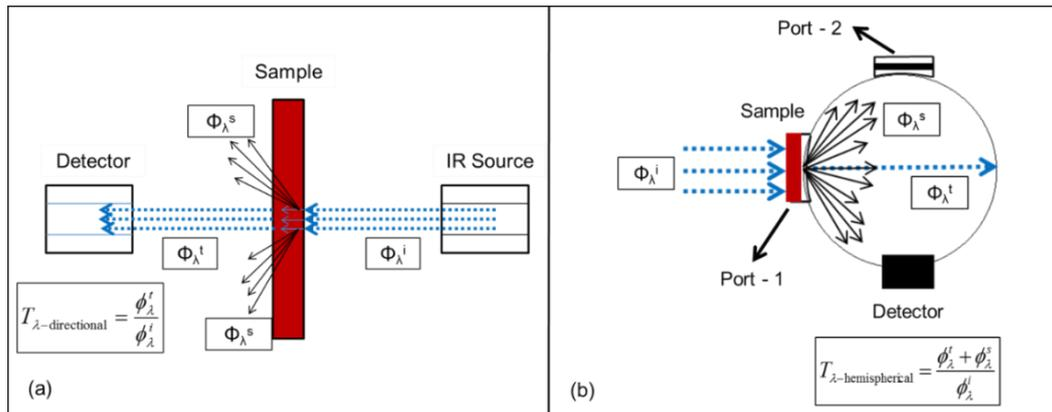
Figure 1: The experimental test set-ups for the bi-directional and directional-hemispherical transmittance measurements of the polymer using FT-IR spectrometer (a) and integrating sphere (b)
