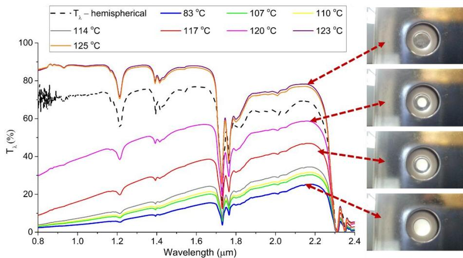
Figure 4: Temperature dependence of the bi-directional transmittance (solid lines) and its comparison to the directional-hemispherical (dashed line) obtained at room temperature
