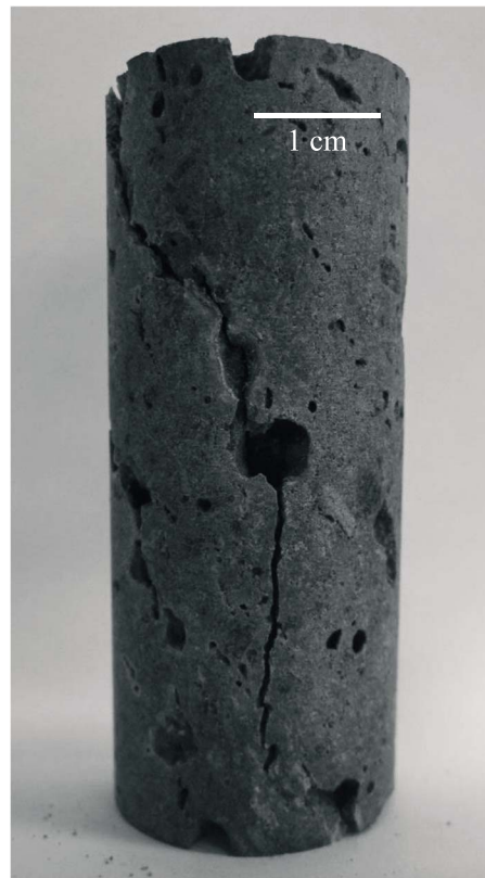
Figure 5. Photograph of the sample BB_2 from block EB_VI deformed uniaxially to failure. Pore-emanated cracking is visible on the surface of the sample.
