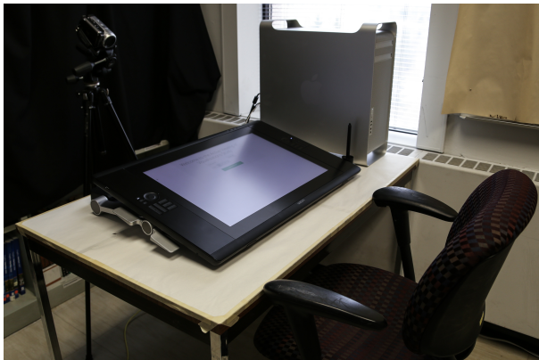
Fig. 9. The physical study setup used a 24 inch pen-and-touch display. A camera captured footage of participants' hands on the display.
