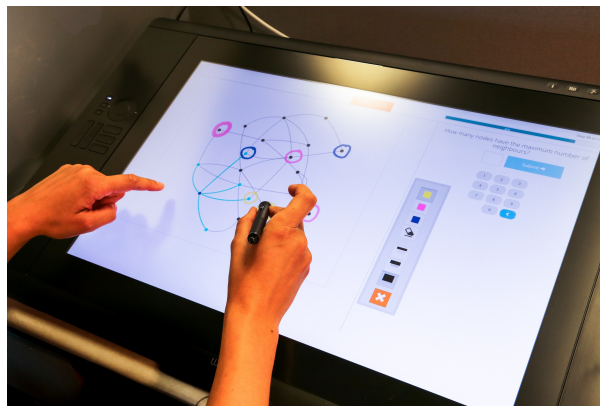
Fig. 8. Using touch interaction to highlight links while highlighting on top of the graph using the freeform annotation overlay.
