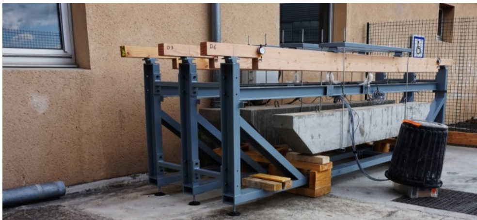
Figure 1: Experimental device use during the creep tests.
