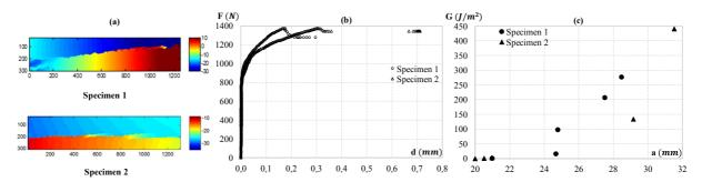
Figure 2: displacement maps (a), force-displacement curves (b), Critical energy release rate (c)
