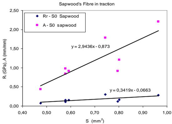
Figure 4 : Evolution curves of rupture strength and rupture deformation of sapwood and heartwood fibers of palmyra according to the cross section
