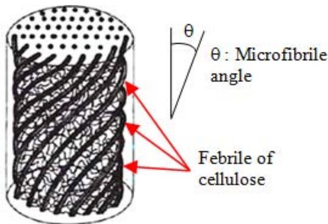
Figure 9 : Model description of the structure of a plant fiber [10]
