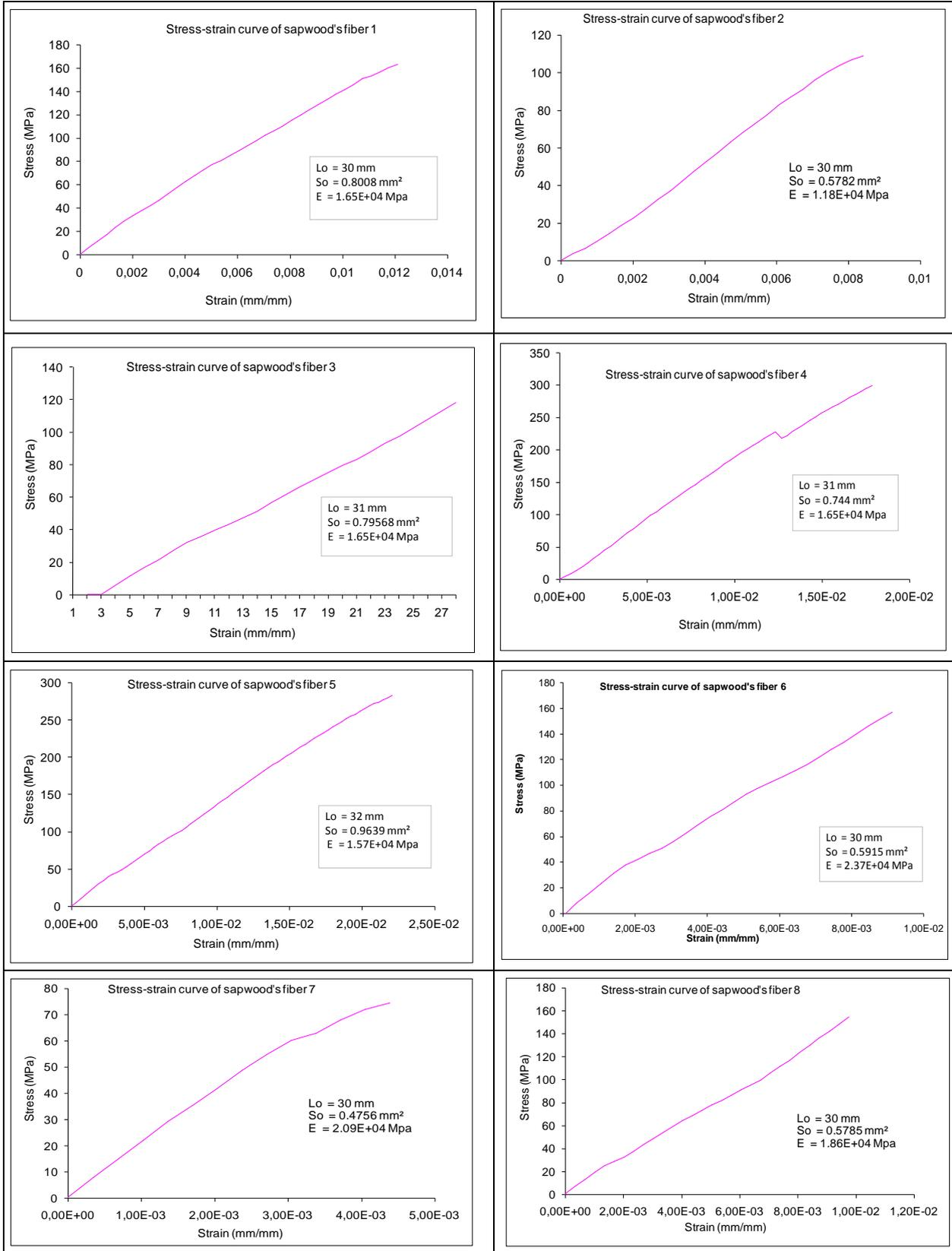
Figure 2 : stress-strain curves of each fiber of the sapwood in traction
