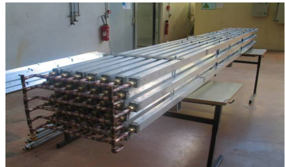
Fig. 4. System of encapsulation of the PCM: tube bank and its device of filling
