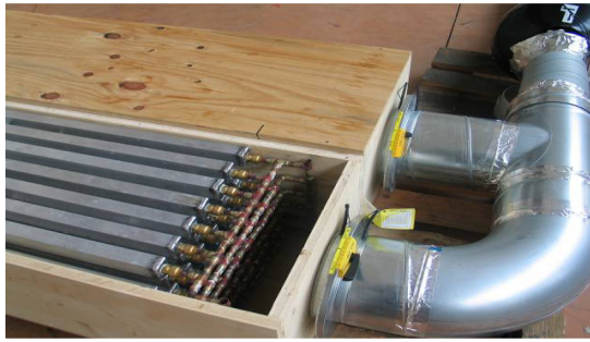
Fig. 5. Associated aerodynamics equipment: system of encapsulation in its box wood, sheath of connection and VMC
