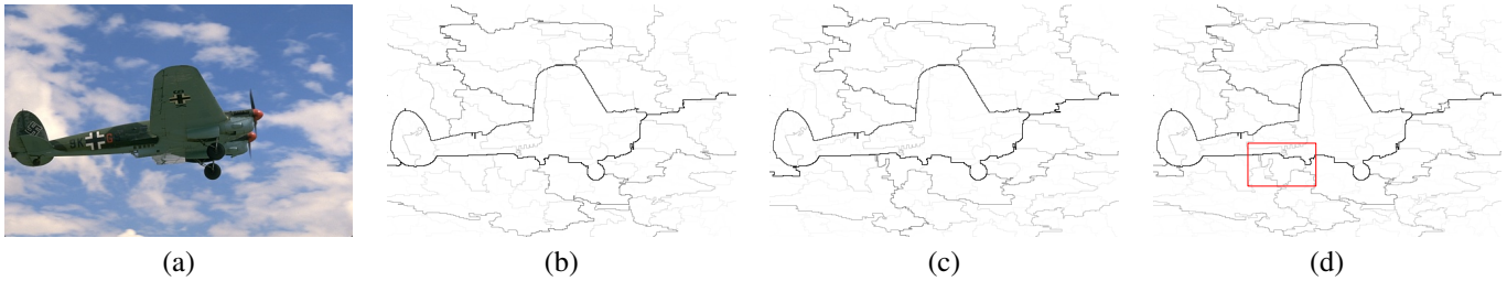
Fig. 2. (a): Original color image; (b): saliency map obtained from (a) with uniform random noise added on the topographic surface; (c): another example of saliency map obtained from (a); and (d) arithmetic average of saliency maps (b) and (c). Details on Fig. (d) show that while the strongest contours of (b) and (c) are preserved due to big ridges on the topographical surface, contours remaining to small catchment basins are slightly different due to the noise disturbance on the topographic surface of the image gradient obtained from (a).
