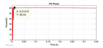
Figure 11. Output power of PV system using MIL test under irradiance change.
