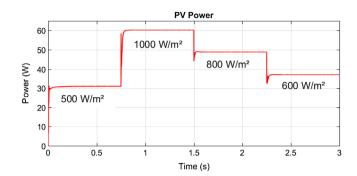
Secondly, the MIL test is made under sudden irradiance variation, Firstly, the solar irradiation is suddenly modified from 500 to 1,000 W/m², and next from 1,000 to 800 W/m², and finally from 800 to 600 W/m². Figure 11 presents the test result, and as shown the modified algorithm presents faster response during irradiance changes and the steady-state oscillations are almost neglected.
