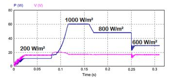
whereas there is a significant PV power variation ( $\Delta P$ ) because the change in irradiance affects PV current instead of PV voltage. Consequently, the  $\Delta P/\Delta V$  steps will be large. Therefore, this moves the operating point far away from the new MPP, which in turn increases the time to reach the new MPP. Therefore, the algorithm efficiency is decreased.
