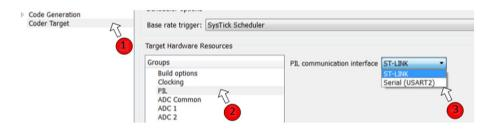
Figure 18. Configure a Simulink model to run PIL.
