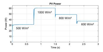
By using PIL test, both Simulink and STM32F4 board will run at the same time and will exchange data based on the modified MPPT algorithm implemented by the PIL block. Therefore, PIL test can be used as a low-cost solution to test the hardware implementation of MPPT algorithm under different conditions of irradiation and temperature.
