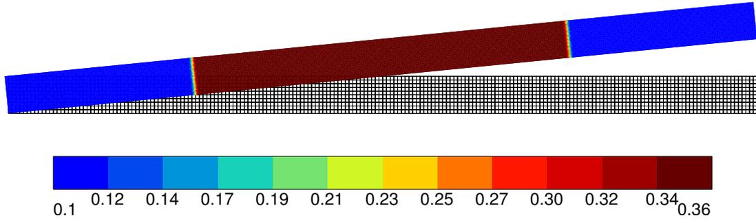
Figure 4: A periodic bigrain structure with superposed rigid body rotation. The color represents the orientation field  $\theta$ .
