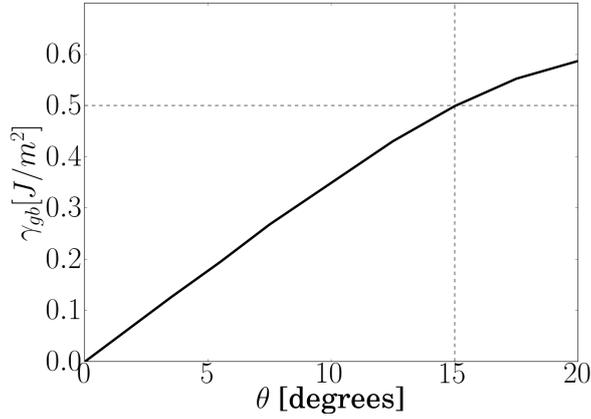
Figure B.12: Grain boundary energies for misorientations up to  $20^\circ$  and  $f_0 = 8.2$  MPa, calibrated to an approximate grain boundary energy of  $0.5 \text{ J/m}^2$  at  $15^\circ$  misorientation.
