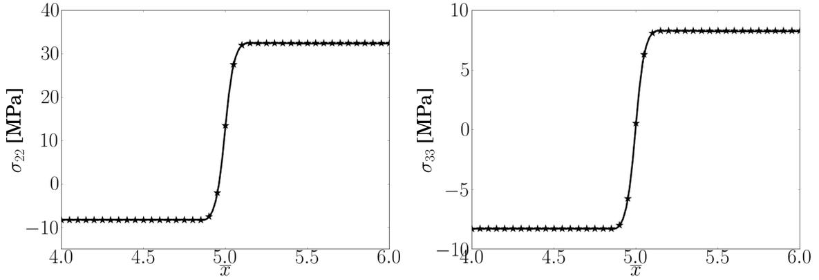
Figure 7: Calculated stress profiles for simple shear loading and anisotropic elasticity. Solid lines show the result from finite element calculations and dashed lines with markers show the analytic solution. Left:  $\sigma_{22}^s$  and right:  $\sigma_{33}^s$  with 1000 finite elements.
