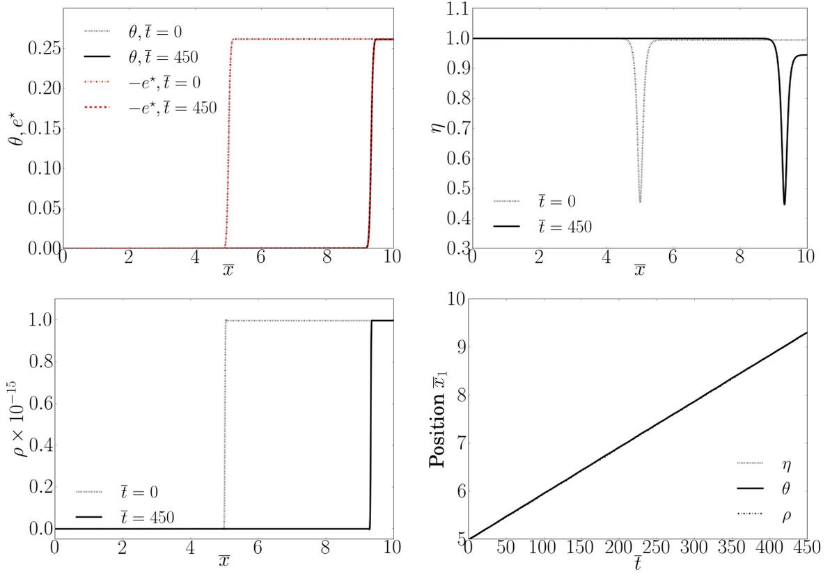
Figure 8: Tracking of the moving grain boundary. Top left and right shows the profiles of  $\theta$  and  $\eta$ , respectively, at  $\bar{t} = 0$  and  $\bar{t} = 450$ . Bottom left shows  $\rho$  at  $\bar{t} = 0$  and  $\bar{t} = 450$ . Bottom right shows the position of the grain boundary (center) over time, for the respective profiles.
