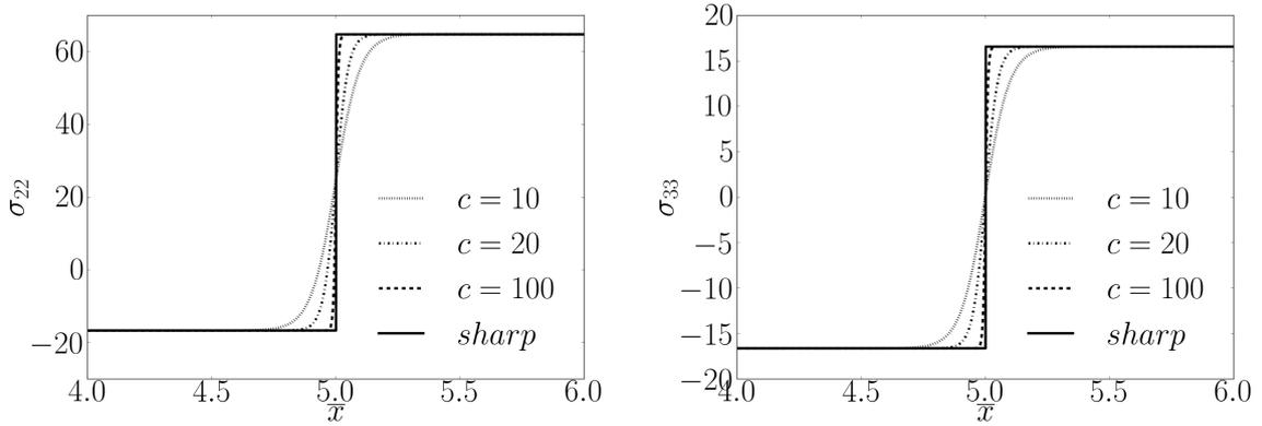
Figure C.13: Analytically resolved stress profiles for pure shear loading and anisotropic elasticity. The solid line is the sharp interface solution and the other lines represent tanh formats of the orientation with increasingly high prefactor.
