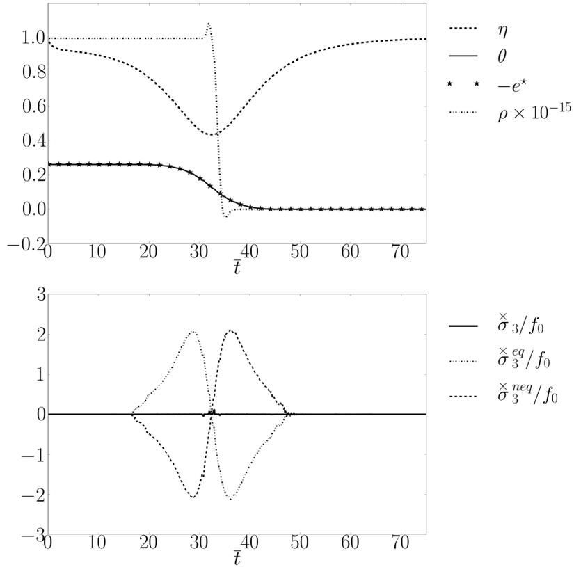
Figure 10: Top: evolution in time of  $\eta$  and  $\theta$  together with  $\rho$  at a fixed point swept by the moving GB. Bottom: evolution in time at a fixed point swept by the moving GB of the skew-symmetric stress  $\check{\sigma}_3^{\times}$  (solid line) and its contributions  $\check{\sigma}_3^{\times eq}$  (dashed-dotted line) and  $\check{\sigma}_3^{\times neq}$  (dashed line), respectively.
