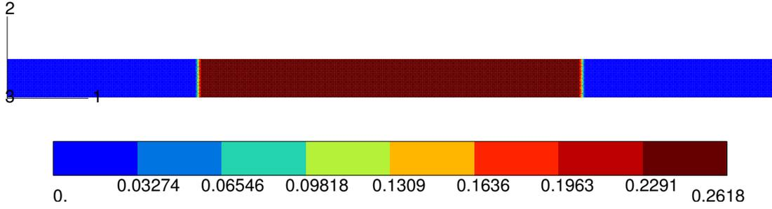
Figure 1: The periodic geometry of the laminated crystal used for simulations, here showing the orientation field  $\theta$  (in rad.). The misorientation is  $15^\circ$ . The microstructure therefore is made of periodically replicated bicrystal layers.
