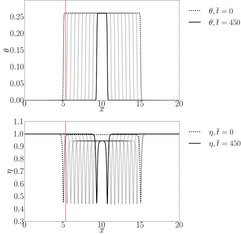
Figure 9: Evolution in time of  $\theta$  and  $\eta$  at discrete time steps  $\Delta\bar{t} = 50$ . The dislocation free grain grows and will eventually annihilate the grain of high stored dislocation density. The red line shows the position of the fixed node where results are extracted over time in figure 10.
