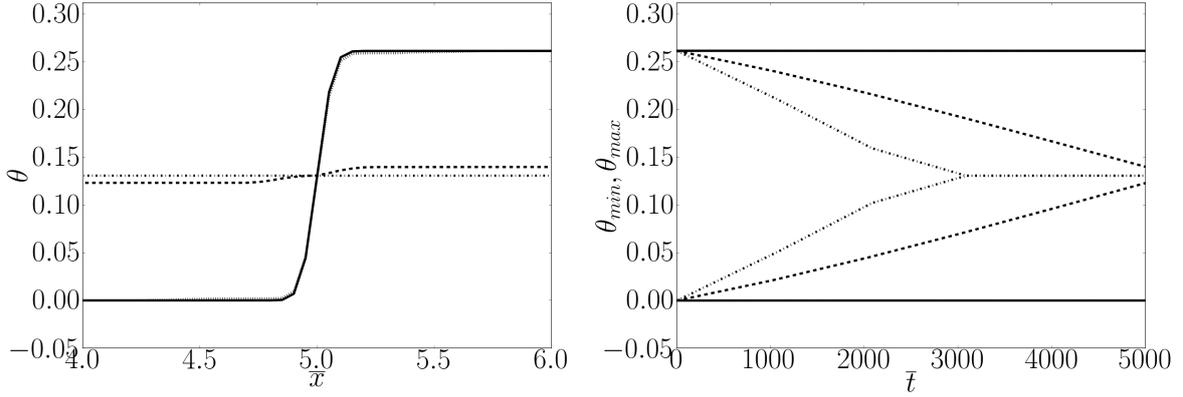
Figure 3: Profiles of  $\theta$  at  $\bar{t} = 5000$  (left) and evolution of  $\theta$  over time (right). Solid line: Cosserat coupling modulus is active (d)  $\mu_c/f_0 = 1000$ . In the other cases, it is not active. Dotted line (a)  $\bar{\mu}_P = 1000$ ,  $\bar{\tau}_\theta = 1000$ . Dashed-dotted line (b):  $\bar{\mu}_P = 0.5$ ,  $\bar{\tau}_\theta = 1000$ . Dashed line (c):  $\bar{\mu}_P = 1000$ ,  $\bar{\tau}_\theta = 1$ .
