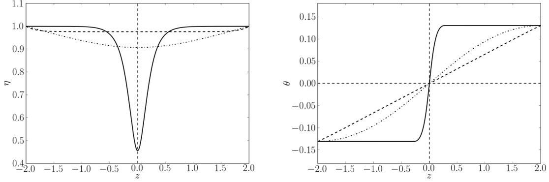
Figure B.11: Profiles for  $\eta^0$  (left) and  $\theta^0$  (right, in rad) for different choices of  $\bar{a}$  and  $\bar{s}$ . Solid lines are for  $\bar{a} = 0.15$  and  $\bar{s} = 0.5$ , the values chosen for calculations. Dashed lines are for  $\bar{a} = 0.15$  and  $\bar{s} = 0.15$  and dashed-dotted lines are for  $\bar{a} = 0.5$  and  $\bar{s} = 0.25$ .
