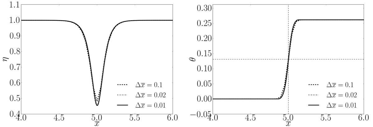
Figure 2: The profiles of  $\eta$  (left) and  $\theta$  (right) at equilibrium for the KWC model. Solid lines: 2000 elements ( $\Delta\bar{x} = 0.01$ ); dashed-dotted lines: 1000 elements ( $\Delta\bar{x} = 0.02$ ) and dashed lines: 200 elements ( $\Delta\bar{x} = 0.1$ ).
