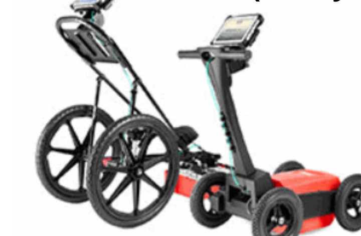
Double frequency 300-800 MHz (UtilityScan DF)
