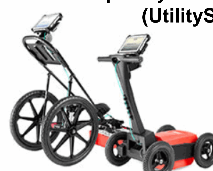
Double frequency 300-800 MHz (UtilityScan DF)
