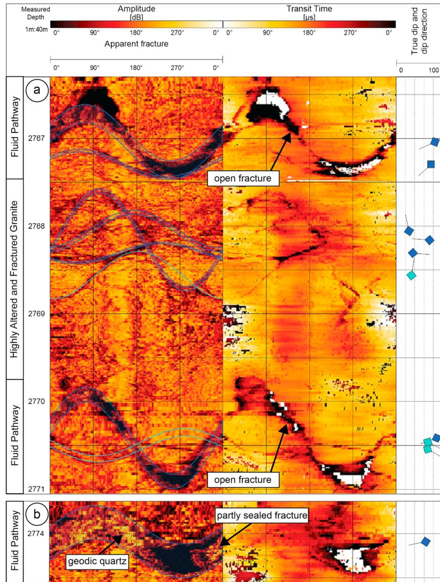
**Figure 10.** Major OP fracture zone affecting the granitic protolith in GRT-2. (a) Major fractures at 2767 and 2770.5 m MD and (b) fracture core at 2774 m MD that characterizes the top of the alteration zone. Colors used for structural interpretation are similar to the legend of Figure 8.
