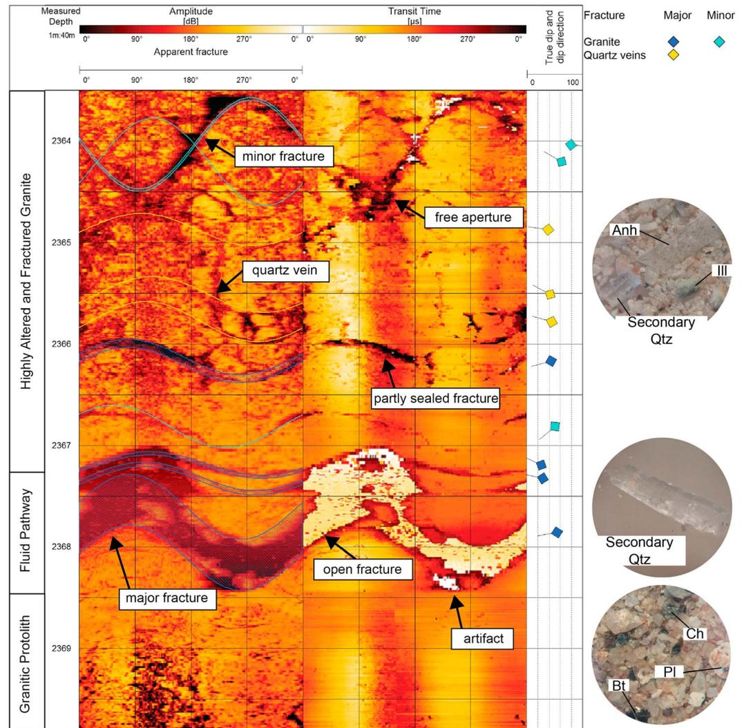
**Figure 2.** Major OP fracture zone affecting the hydrothermally altered granite in GRT-1. Typology used for the structural interpretation is indicated on the acoustic image (light blue = minor fracture, dark blue = major fracture, and yellow = quartz veins). The permeable fracture at 2368 m MD characterizes the limit between the hydrothermally altered granite and the fresh granite.
