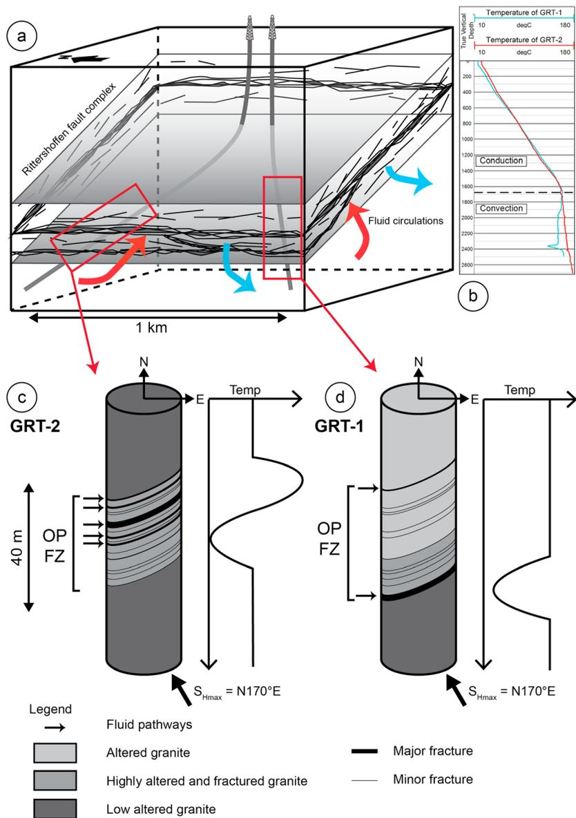
**Figure 14.** Conceptual model of permeable fracture zones in Rittersshoffen wells. (a) Geothermal wells targeted the Rittersshoffen fault zone whose major seismic plane is oriented N-S and dip moderately westward. (b) Temperature profiles indicate a convection zone below the Triassic sediments and in the granitic basement. (c) Schematic section of the major permeable fracture zone in the granite of GRT-2. (d) Schematic section of the major permeable fracture zone in the granite of GRT-1.
