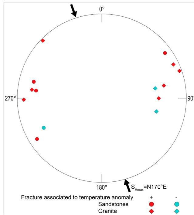
**Figure 12.** Schmidt diagram lower hemisphere of permeable fractures affecting granite and sandstone in GRT-1 and GRT-2. Data are from Table 1. Disks are for fractures in sandstones, diamonds for granite, blue for fractures associated to negative temperature anomaly, and red for positive one.
