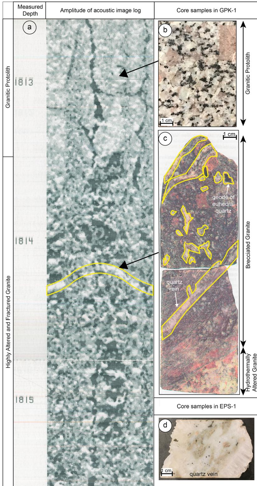
**Figure 3.** Top of a hydrothermally altered fractured zone at 1814 m MD in the geothermal Soultz well GPK-1. (a) Amplitude track of the acoustic image logs, (b) core sample of the granitic protolith, (c) core sample of a silicified zone affected by geodic quartz and transition to the hydrothermally altered granite, and (d) example of quartz vein in a deep permeable fracture zone in EPS-1 Soultz well.
