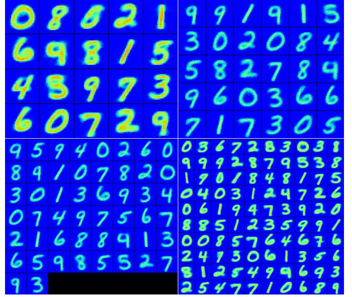
Fig. 5. Sample heat maps of the synaptic weights after network training with four different numbers of output neurons (20, 30, 50 and 100). As it is obvious in the figure, for network using 20 output neurons there is ambiguity in recognition of digits 3, 5 and 8 (underfitting). For networks using more output neurons, we add the number of synapses and network has more chance of learning. In addition, in MNIST testing, we can add the number of neurons to 300 (it is not illustrated in this figure) while still increasing the network prediction ability. However there is limitation of this increment due to overfitting. For instance the network recognition using 500 output neurons is less than network with 300 output neurons.
