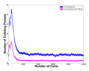
Fig. 6. Number of colliding packets as a function of cycles, OTF with housekeeping and MECB
