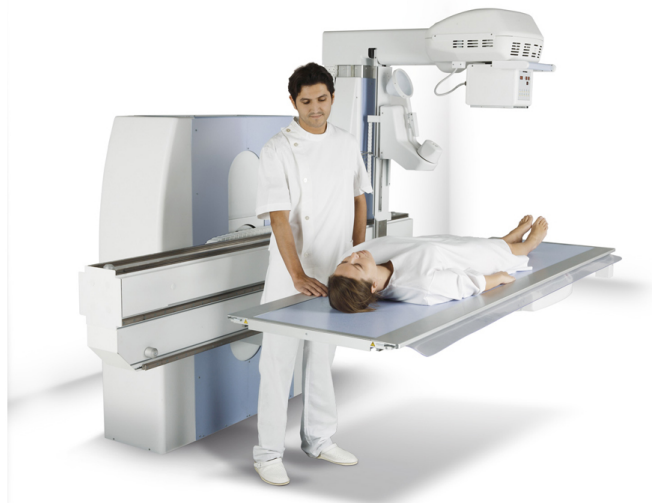
Fig. 1. Example of a radiographic situation with a robotic system carrying a radiation source near a patient and a radiologist. In this situation, unintended collision may arise between the robot and the environment and must be taken into account.
