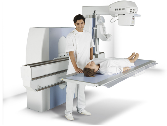
Fig. 1. Example of a radiographic situation with a robotic system carrying a radiation source near a patient and a radiologist. In this situation unintended collision may arise between the robot and the environment and must be taken into account.
