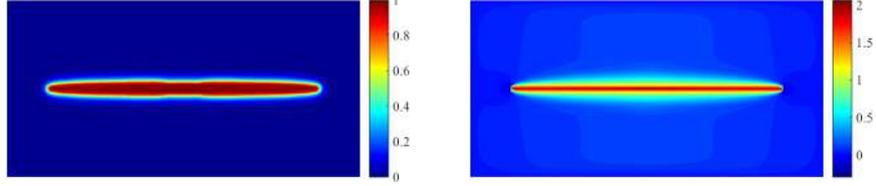
(b) Crack phase field and fluid pressure field with  $k_{\text{homo}} = 2 \times 10^{-14} \text{ m}^2$  at  $t = 16 \text{ s}$ .
