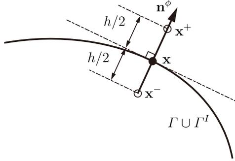
Fig. 2. Approximation of the displacement jump across the interface and the crack.
