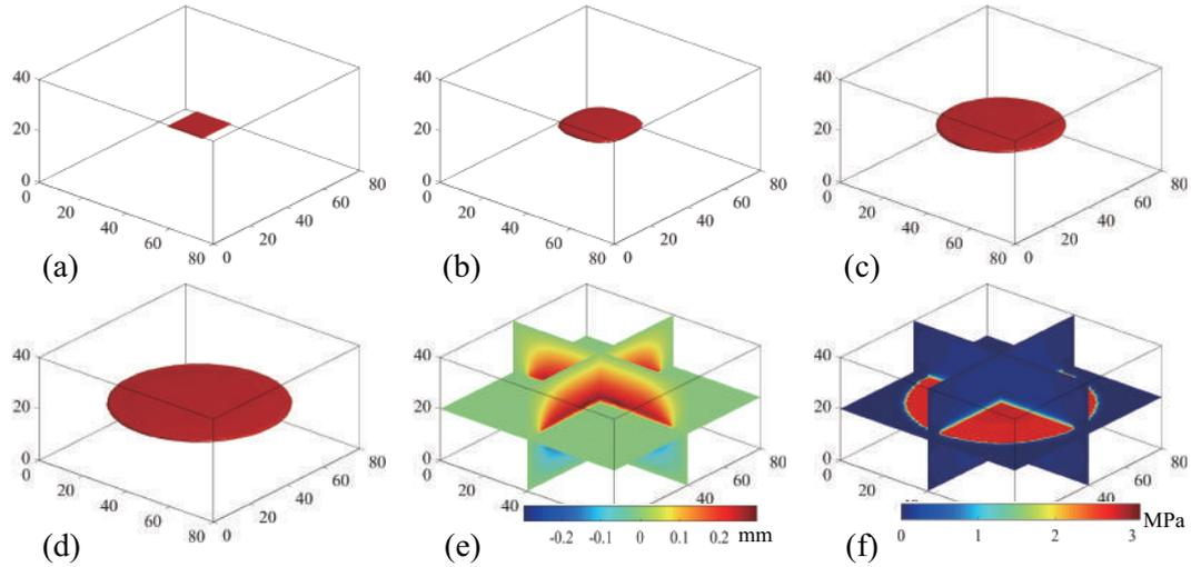
Fig. 18. Hydraulic fracturing simulation of a homogeneous 3D medium subjected to a constant fluid volume injection in the initial crack; crack phase field at (a)  $t = 0$  s, (b)  $t = 2$  s, (c)  $t = 5$  s, (d)  $t = 10$  s; (e) vertical displacement field on selected slices at  $t = 10$  s; and (f) pressure field on two slices at  $t = 10$  s.
