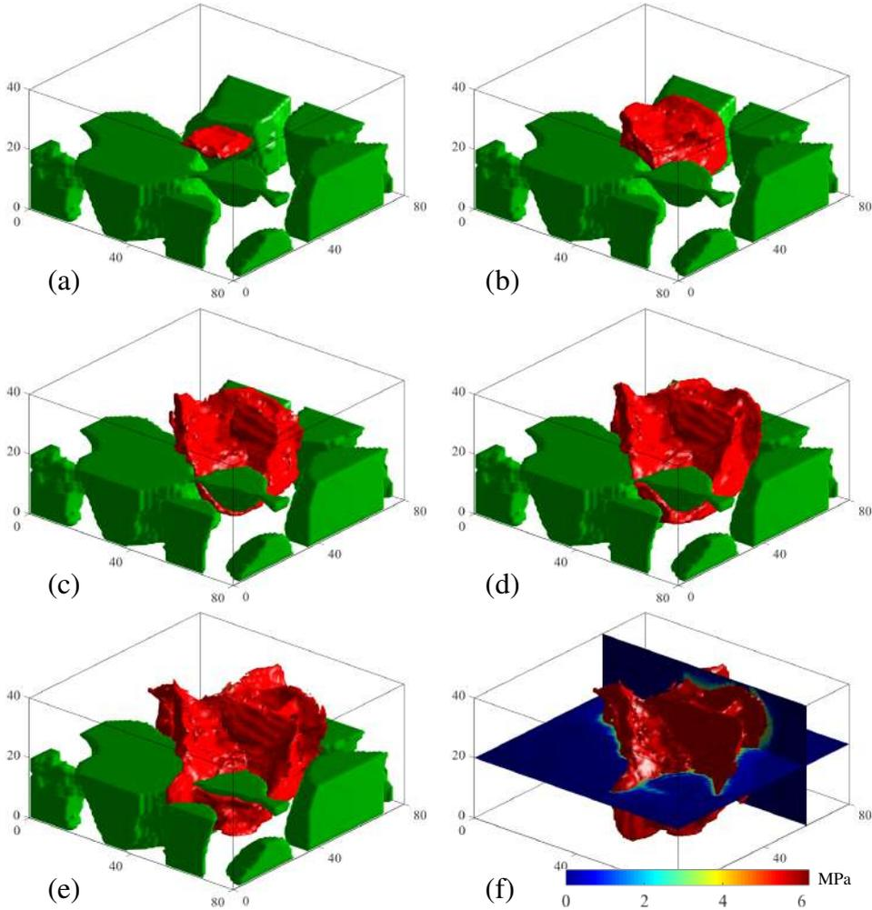
Fig. 21. Evolution of crack phase field during the hydraulic fracturing of the realistic heterogeneous 3D medium at (a)  $t = 1$  s, (b)  $t = 6$  s, (c)  $t = 12$  s, (d)  $t = 18$  s, (e)  $t = 30$  s and (f) pressure field at  $t = 30$ s.
