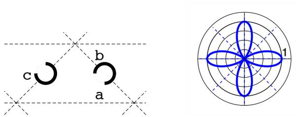
Figure 19: trivial tetragonal flexural lattice material structure and pseudo-Young's modulus
