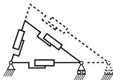
Figure 6: Flexural materials: dilational mode with no rigidity (rectangular boxes represent slide links)
