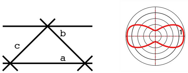
Figure 13: trivial  $R_0$ -orthotropic ( $I4 = 0$ ) isosceles tensional lattice material structure and Young's modulus
