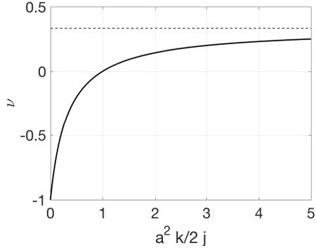
Figure 25: Evolution of Poisson's ratio with respect to the beam properties is case of trivial isotropic material
