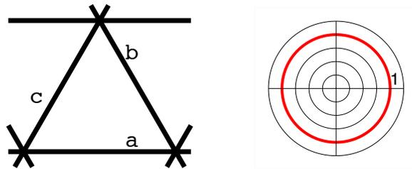
Figure 17: isotropic tensional lattice material structure and Young's modulus
