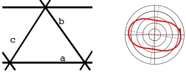
Figure 12:  $R_0$ -orthotropic ( $I4 = 0$ ) tensional lattice material structure and Young's modulus
