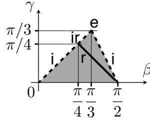
Figure 2: Definition domain of the angles (shaded area) and loci of equilateral (e), isosceles (i), right (r) and right isosceles (ri) triangles.
