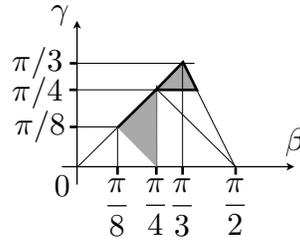
Figure 11: Definition domain of the  $R_0$ -orthotropy (shaded area)
