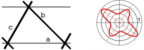
Figure 10: orthotropic tensional lattice material structure and Young's modulus
