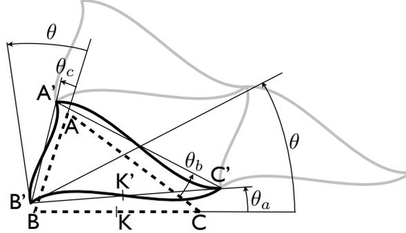
Figure 3: Initial (thick dashed lines) and deformed (thick plain lines) state of a triangular cell and rotation angles
