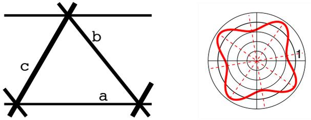
Figure 15: tetragonal tensional lattice material structure and Young's modulus
