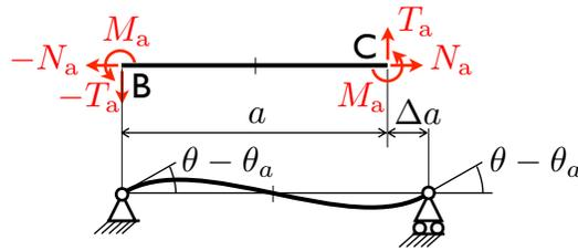
Figure 4: Beam BC. Top: reference geometry and loading. Bottom: kinematics and deformed state
