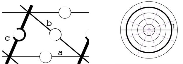
Figure 26: isotropic lattice material structure and Young's modulus
