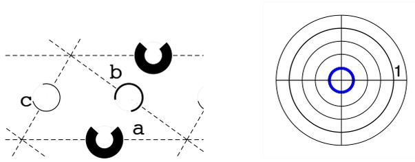
Figure 21: non-trivial isotropic flexural lattice material structure and pseudo-Young's modulus
