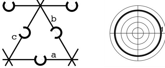
Figure 24: trivial isotropic lattice material structure and Young's modulus
