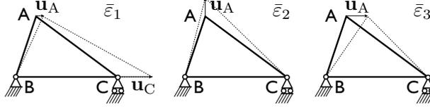
Figure 5: Nodal displacements associated to the elementary strains
