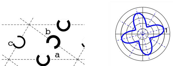
Figure 18: tetragonal flexural lattice material structure and pseudo-Young's modulus
