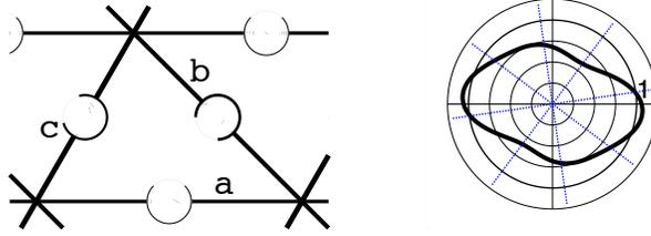
Figure 22: anisotropic lattice material structure and Young's modulus
