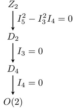
Figure 8: Conditions of appartenance to the 2D symmetry classes of elasticity tensors
