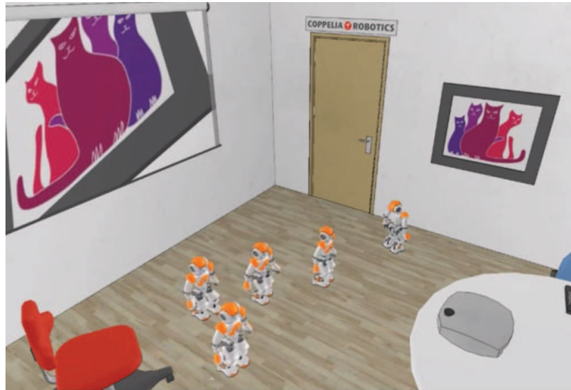
Fig. 4 Multiple NAO humanoids are walking in an office environment in V-Rep. In this scenario, one of the robots' vision is reflected to the projector. Image courtesy of Marc Freese, Coppelia Robotics.
