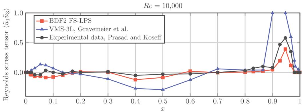
**Fig. 7.**  $\langle \tilde{u}_1 \tilde{u}_3 \rangle$  on the centerlines of the mid-plane  $y = 0.5$  for  $Re = 10,000$  (factor 500).
