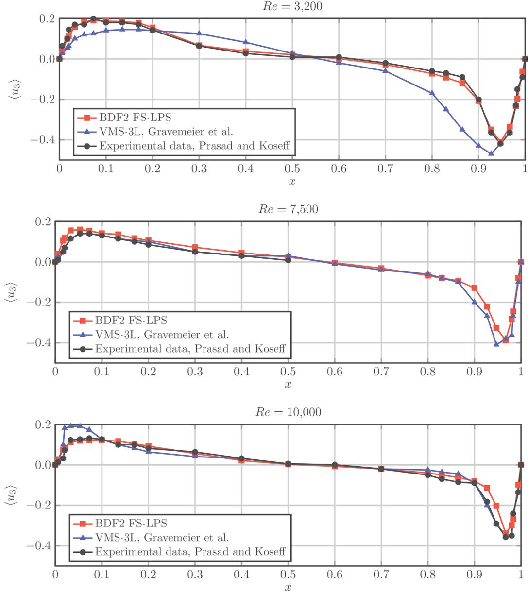
**Fig. 5.**  $\langle u_3 \rangle$  on the horizontal centerline ( $x = 0.5$ ) of the mid-plane  $y = 0.5$  for  $Re = 3,200, 7,500, 10,000$ .
