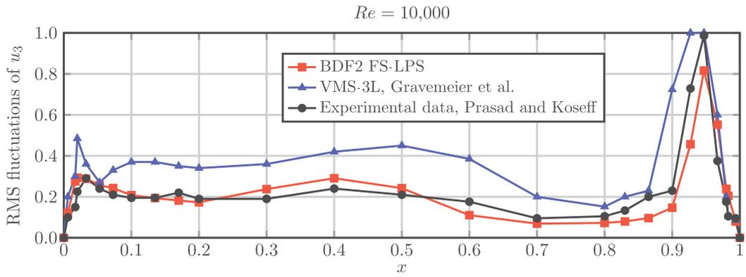
**Fig. 6.**  $\sqrt{\langle \tilde{u}_1^2 \rangle}$  and  $\sqrt{\langle \tilde{u}_3^2 \rangle}$  on the centerlines of the mid-plane  $y = 0.5$  for  $Re = 10,000$  (factor 10).
