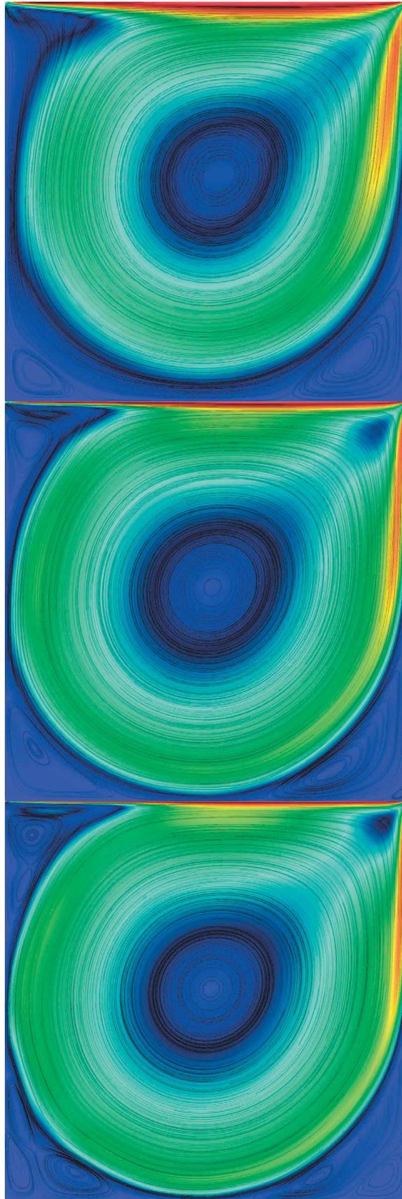
**Fig. 1.** Streamlines on colored velocity distribution at  $Re = 1,000, 5,000, 10,000$  (from top to bottom). (For interpretation of the references to color in this figure legend, the reader is referred to the web version of this article.)
