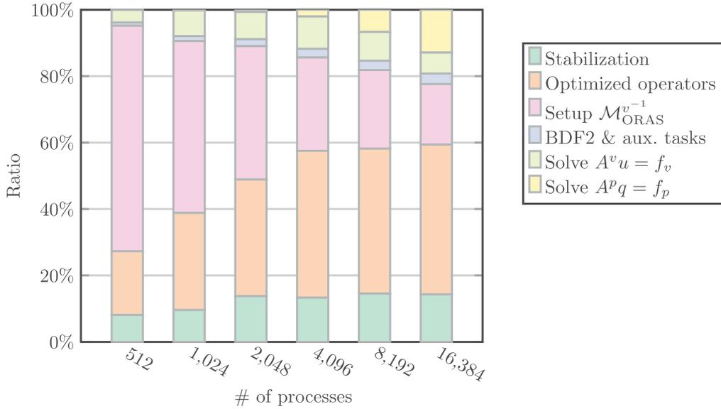
**Fig. 13.** Comparison of the time spent in the various subroutines involved in the scalability analysis of Fig. 11 for a single time step. (For interpretation of the references to color in this figure legend, the reader is referred to the web version of this article.)
