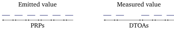
Fig. 3. Illustration of the differences that a signal degradation can make between emitted and measured signals.
