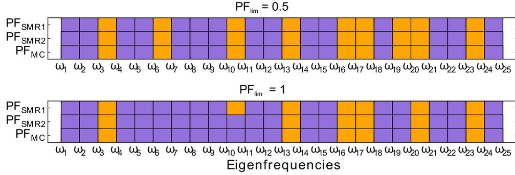
Figure 18: Impact of the limit value of PF on the number of eigenvalues to be refined
