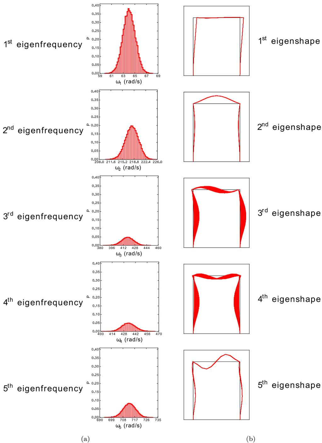
Figure 12: Marginal density of the first 5 random frequencies (a) and the corresponding eigenshapes (b)
