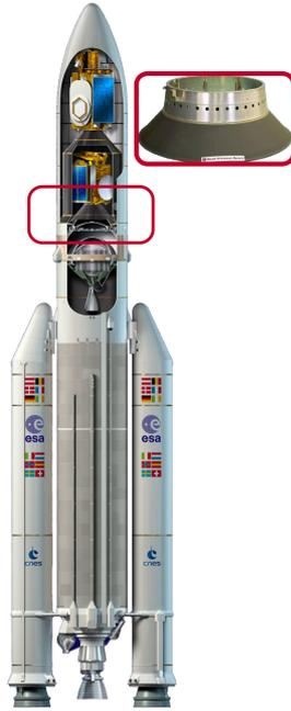
Figure 19: Ariane 5 launcher and one of its payload adapter systems [55]
