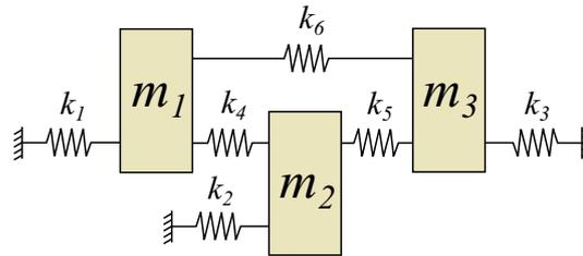
Figure 4: Three-degrees-of-freedom undamped spring-mass random system
