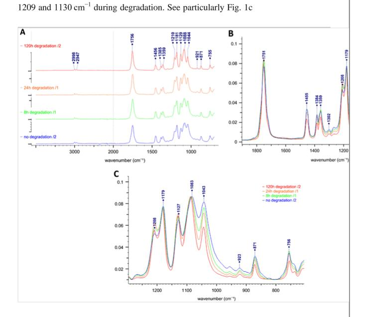
The IR spectra of all PLLA samples, non-degraded and degraded present the common features of PLA polymers formed of L-lactic acid units. In particular, a
