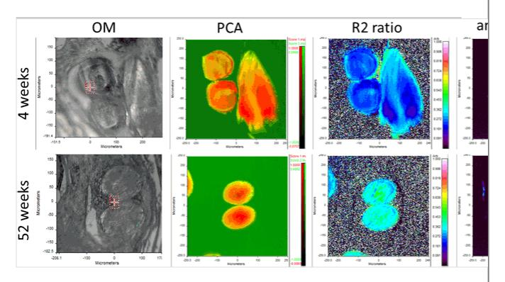
Fifty two weeks after implantation, it was still easy to locate PLLA fibers on both OM pictures and PCA maps and no material breaks or splits could be noticed. This time, however, a crystallinity gradient was observed on the R2 ratio map: a more crystalline (meaning more degraded) area appeared in the central part of each fiber. Even though these differences were still weak, they were in accordance with the current hypotheses on PLLA degradation
