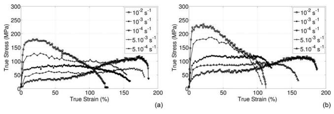
Figure 4. Stress-strain response at T = 700 °C (a) and T = 650 °C (b) for different strain rates (ultrafine grained microstructure)
