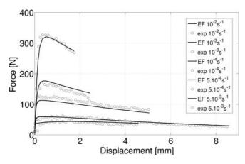
**Figure 7.** Comparison of the Force-displacement response at the scale of the specimen -T = 700 °C for the ultrafine grained microstructure at the end of the Step 3
