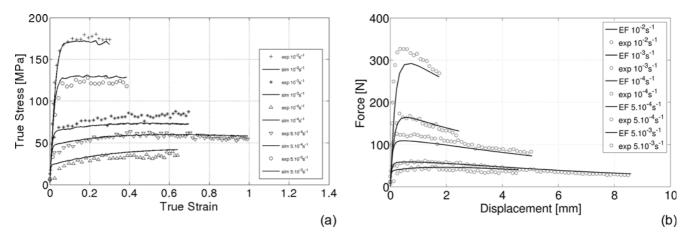
**Figure 6.** Comparison of the stress-strain response provided at the scale of the representative elementary volume (a) and of the Force-displacement response at the scale of the specimen (b) -T = 700 °C for the ultrafine grained microstructure at the end of Step 2.
