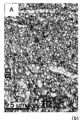
Figure 1. Starting microstructure (a); ultrafine grained microstructure (b)
