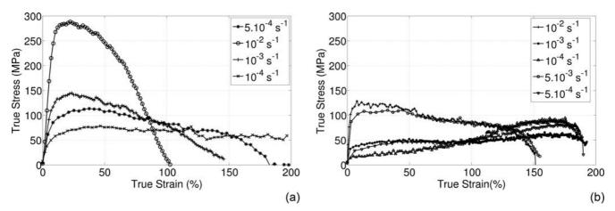
Figure 3. Stress-strain response at T = 750  $^{\circ}$ C and different strain rates for the starting microstructure (a) and the ultrafine grained microstructure (b)
