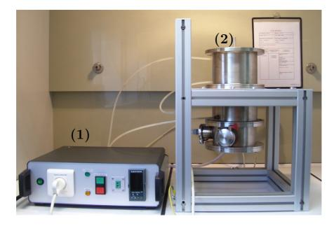
Fig. A.1. Experimental device. (1) power supply, (2) image furnace.
