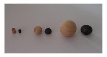
Fig. A.5. Samples before and after exposure. From left to right: 5 mm cylinder, 10 mm sphere and 20 mm sphere.
