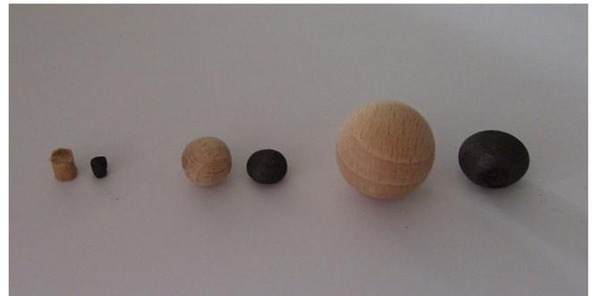
Fig. A.5. Samples before and after exposure. From left to right: 5 mm cylinder, 10 mm sphere and 20 mm sphere.
